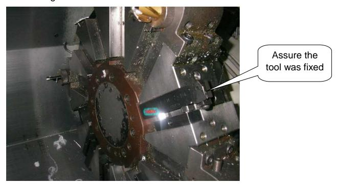
6. Check each tool holder is adequately mounted.
